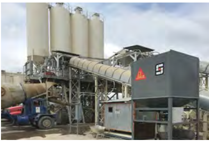
Fig. 8.13.2: Colored concrete demands far more than just adding the pigments. From planning to installation, essential decisions must be made for the application to succeed and the most diverse production steps must be checked and executed expertly. The picture shows a Sika Scofield Granular Color Dispenser at a concrete plant.
