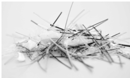
Fig. 8.11.1: Fibers for use in concrete are produced from different materials and qualities of these materials, plus they can have different geometric dimensions and form, according to the required performance of the fresh or hardened concrete.
