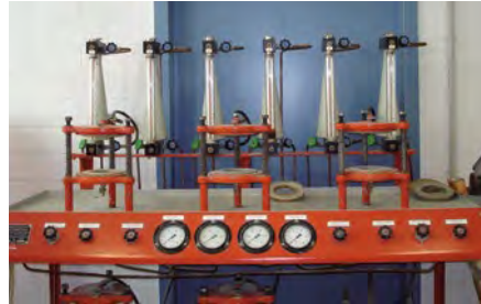
Fig. 8.1.1: Water absorption of concrete under pressure measures the maximum water penetration in mm after a defined time with a specified pressure. (72 hours with 5 bar according EN12390-8)
