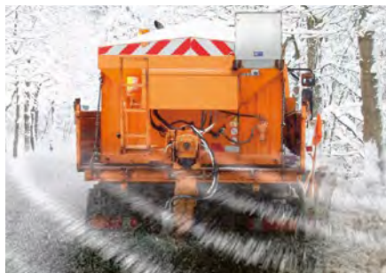
Fig. 8.3.3: Scattered de-icing agent considerably intensifies the reaction upon freezing of water and leads to substantially greater damage in areas of concrete close to the surface.
