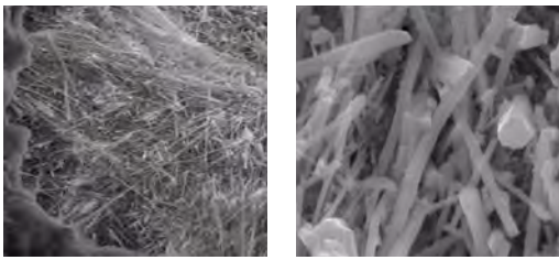
Fig. 8.4.2: Classic form of sulfate attack associated with ettringite or gypsum formation. Flurry of ettringite rods grown in mature cement pastes subjected to external sulfate solutions.
