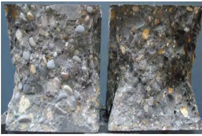
Fig. 8.9.2: The differences in the quality of aggregates and the w/c-ratio determines whether fractures occur in the aggregates or the cementitious paste at the point of maximum loading. The picture shows a reduction of the w/c-ratio from 0.32 (left) down to 0.28 (right).
