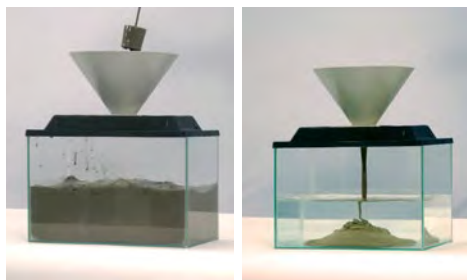
Fig. 8.14.2: Concrete poured underwater with-out (left) and with Sika® Stabilizer UWC (right).
