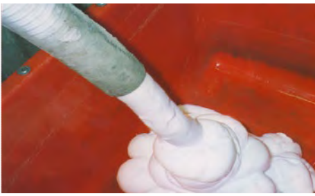
Fig. 8.15.2: Foam generated by a foam generator and Sika®Stabilizer Poro to produce cellular / foam concrete.
